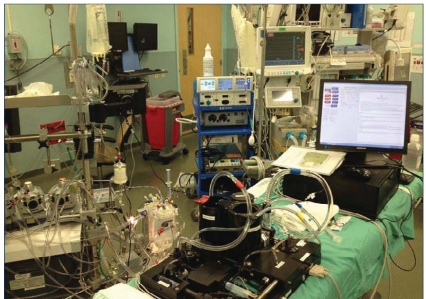
The components of a perfusion simulator include the computer control base, the hydraulic simulator unit with electrocardiogram and a touch pad for the perfusion pump operator. (VA courtesy photo)
